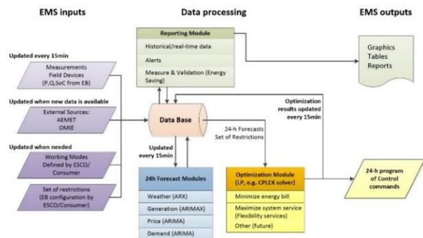
Figure 1. Algorithm data flow in the Spanish demo
