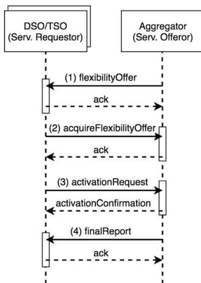
Figure 5. Flexibility B2B sequence diagram
