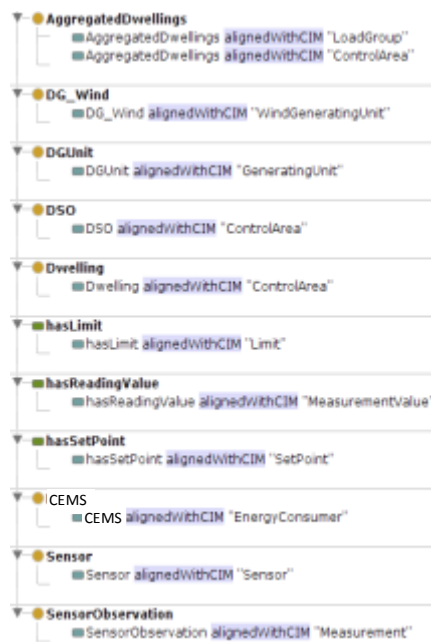
Figure 18 Alignment of ontological concepts with CIM
